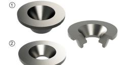
Interchangeable discs for shrink fit chucks with very short A-dimensions (e.g. TBUC) The chuck dips easily into the ferrite disc here. At the same time it is ensured, that the coil does not rest on the collar of the HSK and thus the coil is not damaged when heated.
